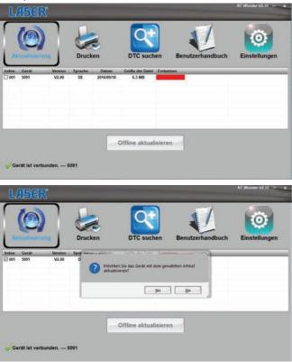
The software update to the 5091 will begin. **Do not disconnect** the 5091 from the computer until the process is complete! On the 5091 the screen will go **GREEN** as the first section completes. **Wait** until the screen goes **BLUE** before restarting the 5091 (**RED** button).
